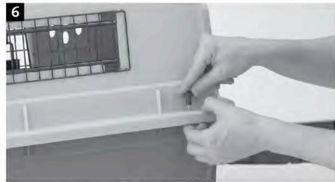
**6.** Insert metal bolt from bottom into square holes and thread on plastic nut. Complete bolt and nut assembly around entire crate.
